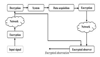
Fig. 1. The structure of the secure observer.
