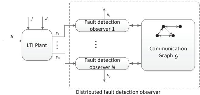
Fig. 1. Framework of distributed fault detection observer
